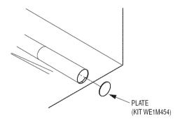
Connect standard metal elbows and ducts to complete the exhaust system. Cover back opening with a plate (Kit WE1M454) available from your local service provider. Place dryer in final location.
