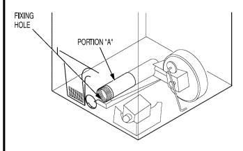
Reconnect the cut portion (A) of the duct to the blower housing. Make sure that the shortened duct is aligned with the tab in the base. Use the screw saved previously to secure the duct in place through the tab on the appliance base.
