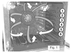
Fig. 1 - Air circulation of Convection Cooking
