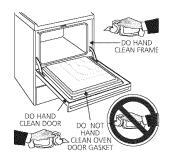
Use soap & water to thoroughly clean the top, sides and front of the oven door. Rinse well. You may use a glass cleaner on the outside glass of the oven door. **DO NOT** immerse the door in water. **DO NOT** spray or allow water or the glass cleaner to enter the door vents. DO NOT use oven cleaners, cleaning powders or any harsh abrasive cleaning materials on the outside of the oven door.
