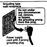
All models are equipped with appropriate 3prong service plug to provide proper service and
