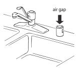
Make sure to use an air gap if the drain hose is connected to house plumbing lower than 20" (50.8 cm) above subfloor or floor.
