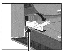
Lock engaged for door removal
