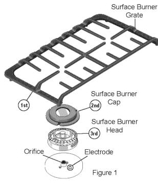
The Grates, Burner Caps and the Large 18k Burner Head should be routinely cleaned. Keeping the burner ports clean will prevent improper ignition and an uneven flame. If needed, the fixed burners should be cleaned in place with an humid cloth (do not spraw water on them).
