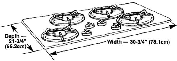
30" (76.2cm) min. base cabinet is required. If cabinet has a drawer, a 3-1/2" (8.9cm) depth clearance from the countertop to the top of the drawer (or other obstruction) in base cabinet is required.
