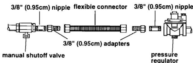
All connections must be wrench-tightened.
