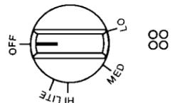
burners. Push in and turn each control knob to "LITE" position. The flame should light within 4 seconds. Do Not leave the knob in the "LITE" position after burner lights.
