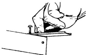
**5.** Attach the mounting brackets to each side of the burner box with the 5/16" (0.80cm) screws. Do Not tighten the screws. Turn the mounting brackets so each is under the burner box.
