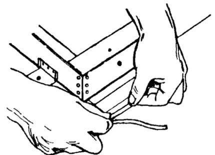
**3.** Remove the paper backing from a small section of the foam sealing strip. Place the strip 1/8" (0.3cm) from cooktop edge on the underside of the glass. Continue until foam strip completely outlines the edge of the cooktop. Do Not use additional sealant around outer edge of cooktop.
