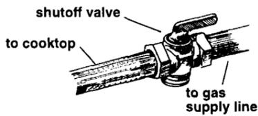
**F.** The supply line shall be equipped with an approved shutoff valve. This valve should be located in the same room as the cooktop and should be in a location that allows ease of opening and closing. Do Not block access to shutoff valve. The valve is for turning on or shutting off gas to the appliance.
