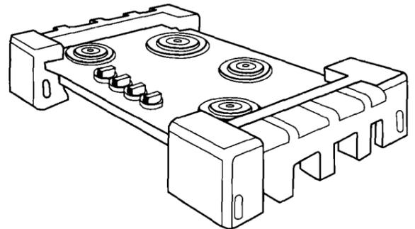
**1.** Remove shipping materials and tape from cooktop. Remove pressure regulator and hardware package from side of carton. Write down the model and serial numbers on the front of these instructions before installing the cooktop. The numbers are on the model/serial rating plate located on the bottom of the cooktop burner box.
