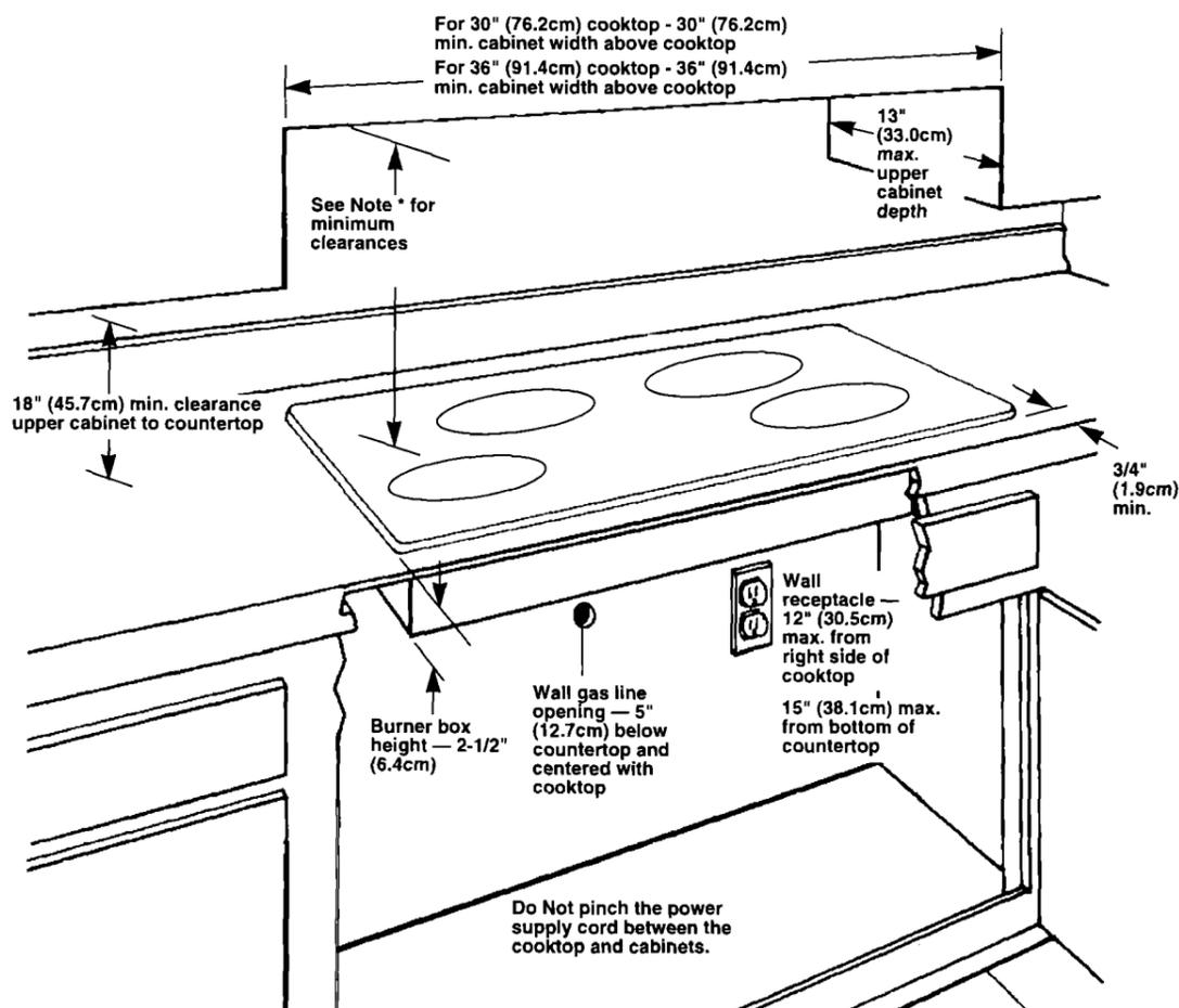
\* Note: 30" (76.2cm) min. when bottom of wood or metal cabinet is protected by not less than 1/4" (.6cm) flame retardant millboard covered with not less than No. 28 MSG sheet steel, 0.015" (.04cm) stainless steel, 0.024" (.06cm) aluminum or 0.020" (.05cm) copper.
