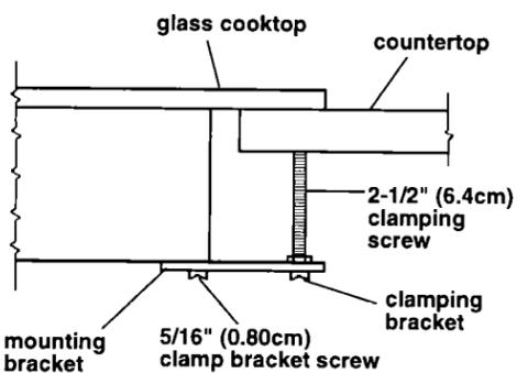
**7.** Rotate mounting brackets away from burner box. Tighten the mounting brackets to the burner box. Insert the 2-1/2" (6.4cm) clamping screws into the mounting brackets. Use a screwdriver to tighten screws against the underside of countertop.
