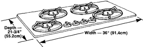
36" (91.4cm) min. base cabinet is required. If cabinet has a drawer, a 3-1/2" (8.9cm) depth clearance from the countertop to the top of the drawer (or other obstruction) in base cabinet is required.
