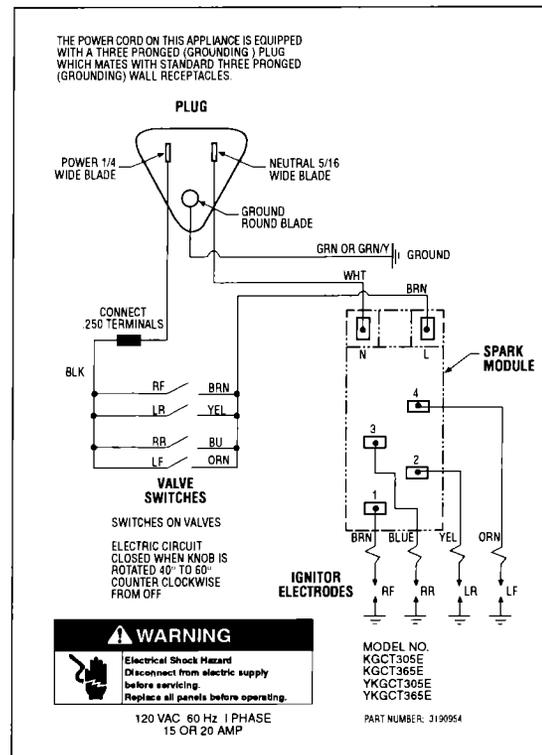
The power cord on this appliance is equipped with a three-pronged (grounding) plug which mates with standard three-pronged (grounded) wall receptacles.
