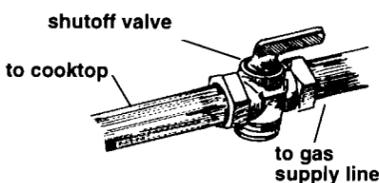
**11.** Open the shutoff valve in the gas supply line. Wait a few minutes for gas to move through the gas line.
