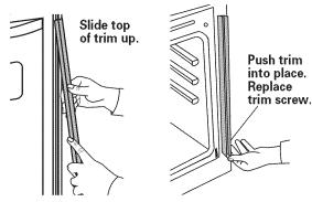
Slide top end of each trim upward onto oven side rails. Push each trim into place at bottom of trim. Use screws to attach each trim to oven. Take care not to scratch other surfaces with ends of trim.
