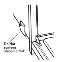
Turn power supply off. Move oven close to final position.
