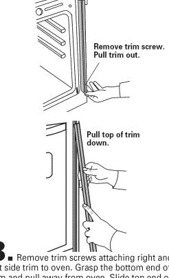
Remove trim screws attaching right and left side trim to oven. Grasp the bottom end of trim and pull away from oven. Slide top end of trim downward to remove trim from oven. Take care not to scratch other surfaces with ends of trim. Set trim and screws aside on protected surface.
