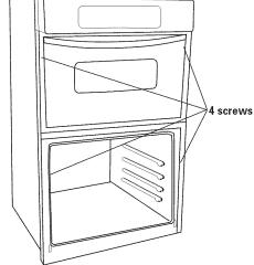
Important: Securely fasten oven to cabinet using the screws provided (two screws for a single oven or four screws for a double oven). Insert the screws through holes in mounting rails. Do Not overtighten screws.
