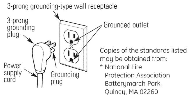
To minimize possible shock hazard, the cord must be plugged into the proper mating three-prong grounding-type wall receptacle, grounded in accordance with the National Electrical Code ANSI/NFPA70—latest edition\* and all local codes and ordinances.
