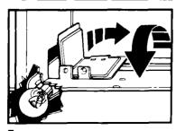
Slide bulb holder out, then turn towards front to remove bulb from oven.
