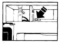
**4.** Remove bulb holder mounting screw.
