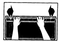
8. Slide the top of the vent cover into place. Push the bottom until it snaps into place. Replace the mounting screws. Turn the power back on at main power supply.
