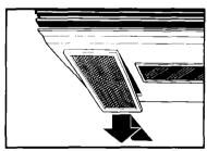
2. To remove grease filters, slide each filter to the front.
