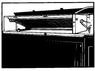
Slide a new charcoal filter into place. The filter should rest at the angle shown.
