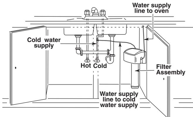
2. Attach the supplied water filter mounting ring and screw at the recommended location.
