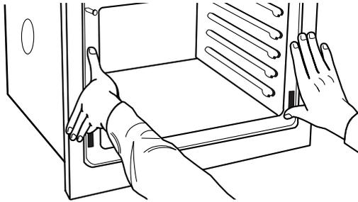
3. Push oven completely into cabinet and center oven into cabinet cutout.
