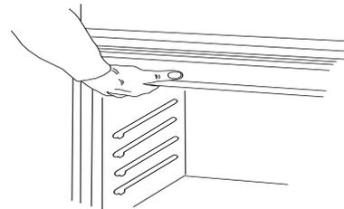
2. Push against seal area of front frame to push oven into cabinet.
