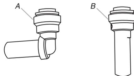
A. Quick connect elbow adapter fitting
