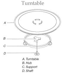
The turntable rotates in both directions to help cook food more evenly. For best cooking results, do not operate the microwave oven without having the turntable in place. See "Assistance or Service" to reorder any of the parts.
