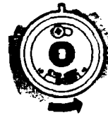
4. To raise the temperature, move black part of knob closer to HI. Each notch equals about 10 F (5 C)
