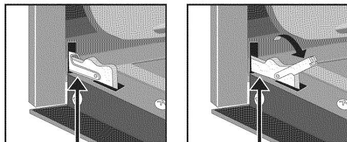
Lock engaged for door removal
