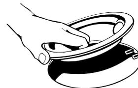
2. Holding the coil element as level as possible, carefully push coil element terminal into the receptacle.
