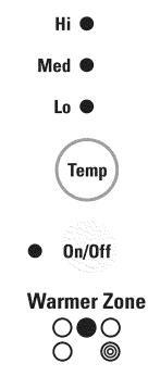
Fig, 1 - Warmer Zone control on backguard
