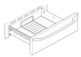
Fig. 2 - Warmer drawer rack in downward position.
