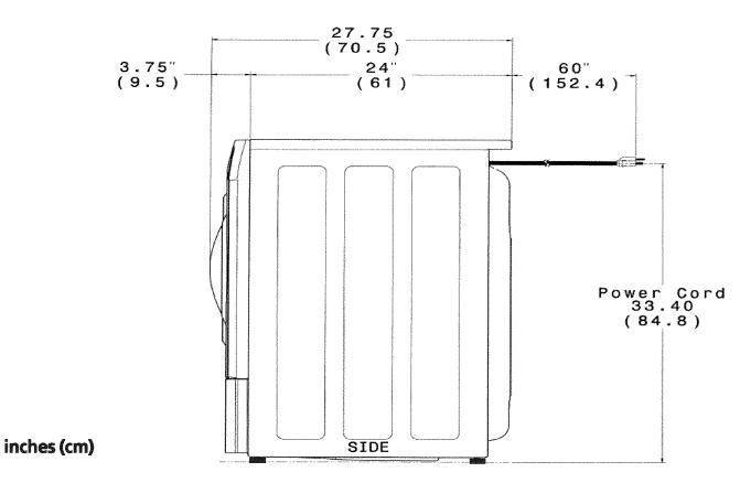
NOTE: For <u>pedestal</u> installations, see additional installation instructions included with the pedestal. For <u>stacking</u> installations, see additional installtion instructions included with the stacking kit. For <u>under counter</u> installations, no special top is required.
