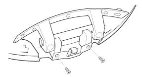
Hold the door on its side with one hand and fasten the remaining 2 screws as shown. Then tighten the 2 screws (#8) holding the hinge assembly.
