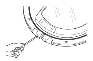
9. Remove the 2 nuts, washers, and the 2 machine screws (#8).
