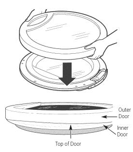
19. After reversing door, there will be a mismatch between the outer door and the inner door.
