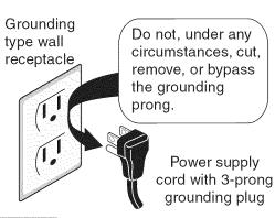
**A WARNING** Avoid fire hazard or electrical shock. **DO NOT** use an adapter plug, an extension cord, or remove grounding prong from electrical power cord. Failure to follow this warning can cause serious injury, fire or death.
