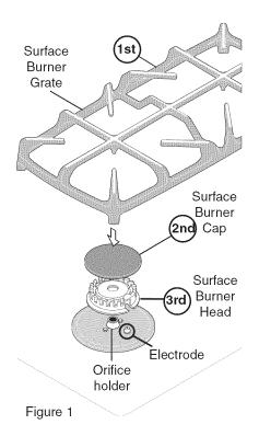
**To Remove and Replace the Surface Burner Caps and Burner Heads -**Remove in the following order: (1st) surface Burner Grates, (2nd) Burner Caps and (3rd) Burner Heads. Replace them in reverse order: Heads, Caps, then Grates.
