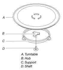
The turntable rotates in both directions to help cook food more evenly. For best cooking results, do not operate the microwave oven without having the turntable in place. See "Assistance or Service" to reorder any of the parts.
