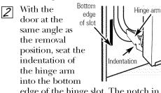
edge of the hinge slot. The notch in the hinge arm must be fully seated into the bottom of the slot.
