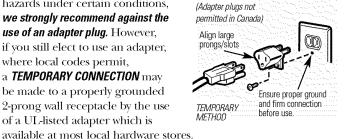
The larger slot in the adapter must be aligned with the larger slot in the wall receptacle to provide proper polarity in the connection of the power cord.
