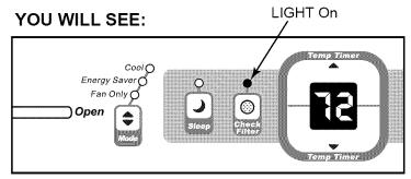
Note: This feature is a reminder to clean the Air Filter (See Care and Cleaning) for more efficient operation and cooling. The LED (light) will illuminate after 250 hours of operation. To reset after cleaning the filter, press the "Check Filter" button and the light will go off.
