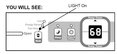
Note: Use this function only when cooling is not desired, such as for room air circulation or to exhaust stale air (Remember to open the vent during this function, but keep it closed during cooling for maximum cooling efficiency). You can choose any fan speed you prefer.
