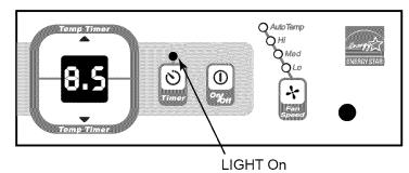
Note: For Delay Stop, the unit must be in the On position. Note: For Delay Start, the unit must be in the Off position.
