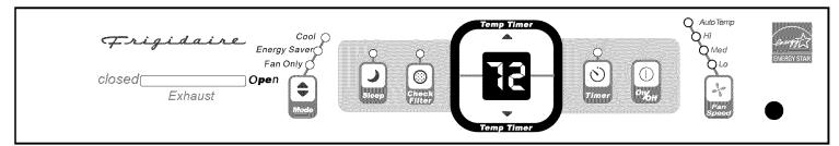
This Exhaust Control allows the air conditioner to either recirculate inside air (CLOSED) or exhaust air to the outside (OPEN). The CLOSED position is used when maximum cooling is desired. It may also be used for air recirculation without cooling when the air conditioner is set in any FAN position.
