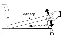
range top, grasp the sides with finger-tips only. Be careful not to pinch fingers. **DO NOT** drop or bend the range top when raising or lowering. This could damage the surface.
