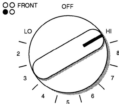
**13. Check the operation of the cooktop elements:** Push in and turn each surface unit control knob to "HI" position. Check the operation of the cooktop elements and indicator lights.
