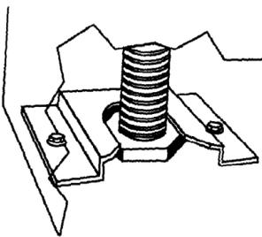
9. Check that rear leveling leg is engaged in anti-tip bracket.
