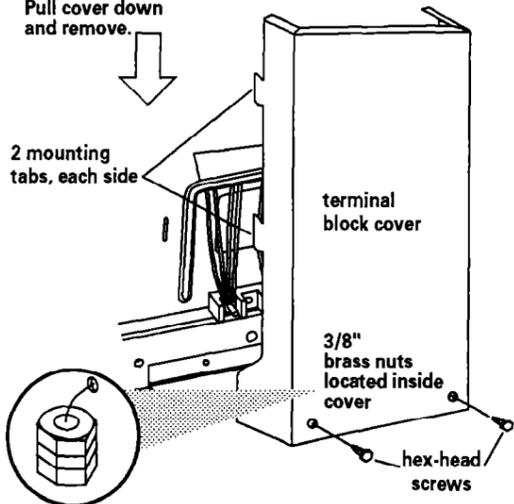
**6** Remove the terminal block cover screws located on the back of range. Pull cover down and towards you to remove cover from range.
