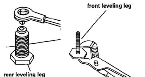
**3.** Remove storage drawer. Use a 3/8" drive ratchet to lower rear leveling legs one-half turn. Use channel lock pliers to lower front leveling legs one-half turn.
