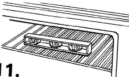
11. Place rack in oven. Place level on rack, first side to side; then front to back.
